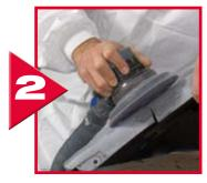
Prepare the area around the crack using a 3M™ Hookit™ Abrasive Disc P80 (for hard plastics) or P180. Avoid overheating and melting the plastic.
