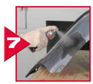
Spray Polyolefin Adhesion Promotor 05917 on the front side of the bumper around the cracked area. Allow 10 minutes to dry.
