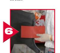
Cut the 3M™ Automix™ Instant Plastic Repair Patch 05888 to size (at least 2-3cm larger than the repair area) and place firmly over the entire crack on the back side of the bumper.
