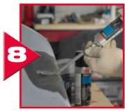
Using 3M<sup>™</sup> Applicator 08190 apply 3M<sup>™</sup> Flexible Parts Repair Material 05901 to the cracked area.
