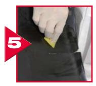
To achieve maximum adhesion use 3M™ Automix™ Patch Adhesion Promoter 06396 to the back side of the repair. Allow 5 minutes to dry.
