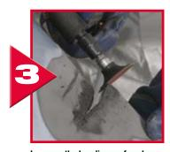
Increase the bonding surface by opening out the crack using a 3M<sup>™</sup> Roloc Disc P80. For a crack reaching the dge of the panel, open the end to make a 'V' shape. Remove plastic residue with a sharp knife.
